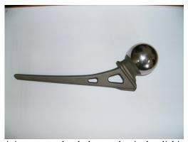
Fig. 1. Artificial hip joint prepared only by mechanical polishing of the surface.
