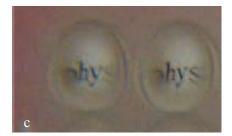
**Fig. 2.** Photograph's of the TESG layer: a) crystallized; b) crystallized microlens; c) chemically processed TESG microlenses (each producing an image of a text**-phy** placed behind the lenses)
