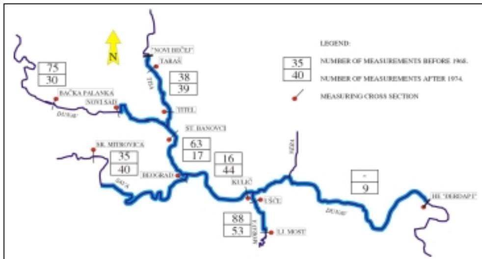
Fig 2: Sediment measuring profiles in the "Iron Gate I" reservoir
