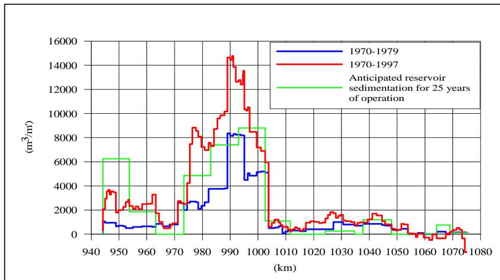
**Fig. 5: Distribution of riverbed changes along the reservoir**
