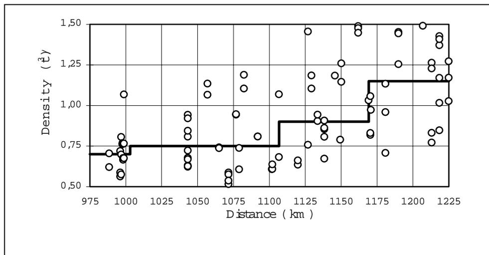
**Fig. 6: Bulk density of sediment deposits**
